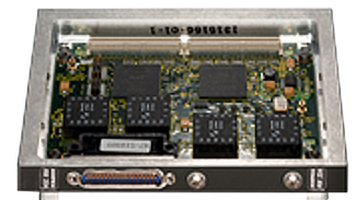
Typical Input Module (AM-204: MIL-STD-1553)
