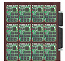
Storage Tray Layout (Heat Dissipation Covers removed)
