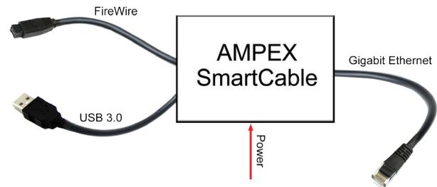
Physically, the SmartCable uses attached data cables, so it can be considered as a cable with an Ethernet jack on one end, a USB or FireWire plug on the other, and a “bump” in the middle. Power to the device is via a wide-input DC supply, supporting both 12V and 28V sources.
